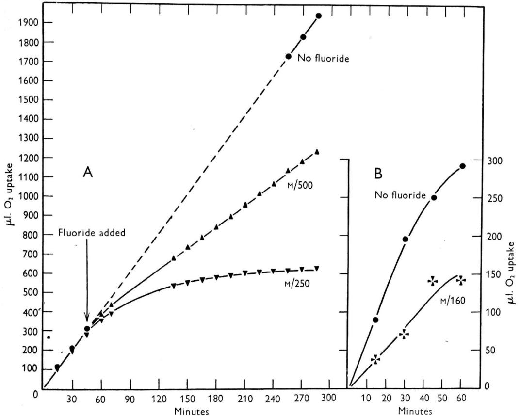
Fig. 9. Effect of fluoride on oxygen uptake. A, spadix slices of *Arum italicum*, fluoride added as shown by arrow. B, extract from spadix of *A. italicum*, fluoride present from start.
